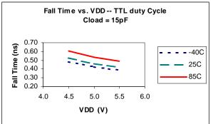
Rise/Fall time vs. Output Loads over Temperatures
