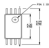
DIMENSIONS IN MILLIMETERS. MIN. MAX.
